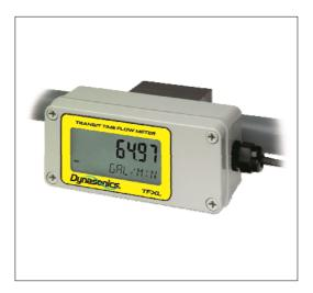
Designed to replace mechanical flow meters where liquid conditions tend to damage or impede operation. Low cost non-intrusive system clamps on the outside of the pipe requiring no maintenance. All meters provide two flow rate outputs: 4-20mA analog and 0-1,000 Hz rate pulse, permitting it to interface with a variety of monitoring equipment. *ULTRALINK* Windows®-based software utility allows users to configure, calibrate and troubleshoot.
